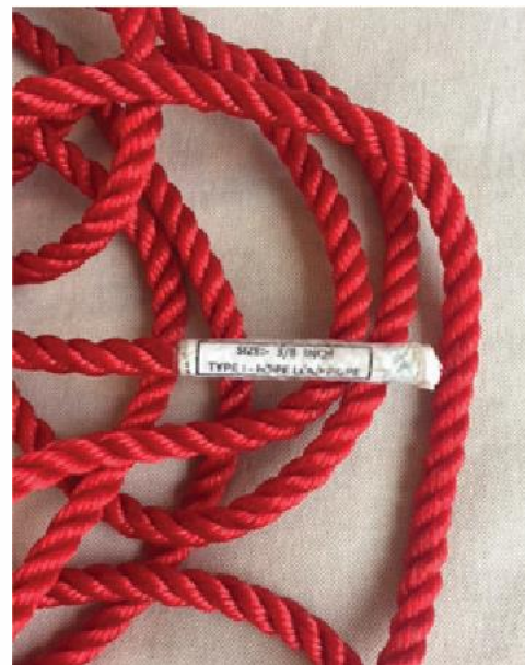
3/8 inch red ‘weak’ rope made by Tufropes Pvt Ltd., India and distributed by Enterprise Shippagan, NB
