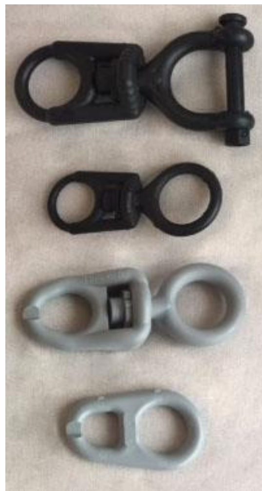
Figure 1. A selection of plastic weak links used in US fixed gear fisheries. The upper left link breaks at 1,500 lb and the other three at 600 lb. The lower most is a flat, non-swivel version.
